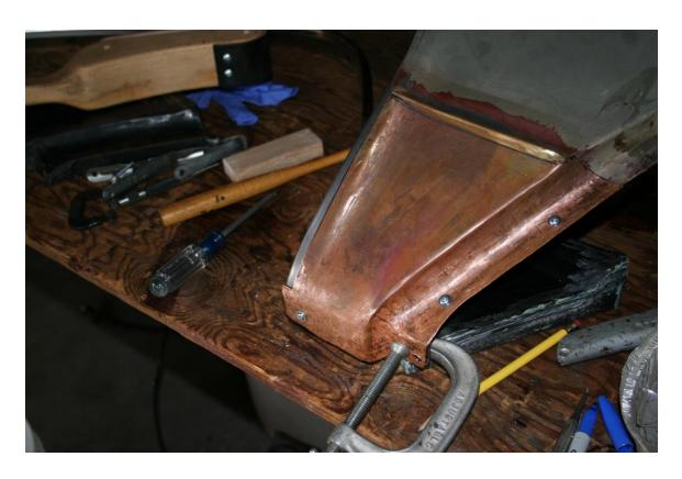
To form the needed piece I tried a brass plate, but could not get it to bend enough to fit the fender. I could not anneal the plate and make it soft enough to work. I anneal a copper plate and it worked out very well. By using a slapper and the English wheel I was able to make the part. Next I had to modify the brass trim part that was on top of this plate. All holes were drilled and the parts installed on the fender.
