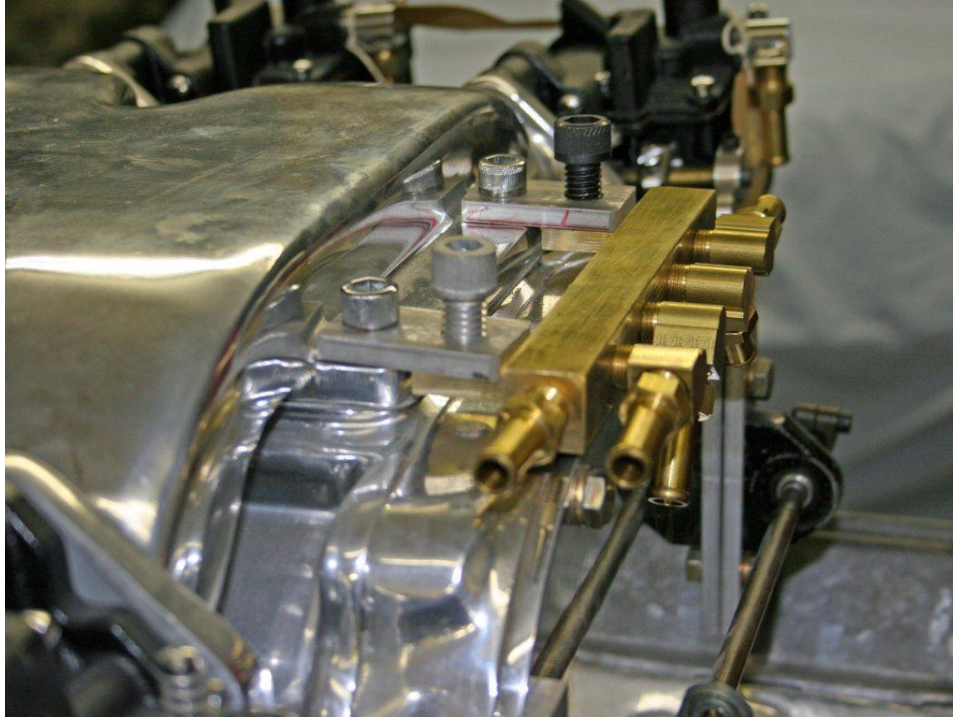
Fuel supply block on rear of blower.
