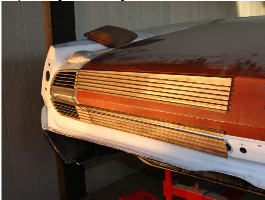
Fit up of casting after machining
