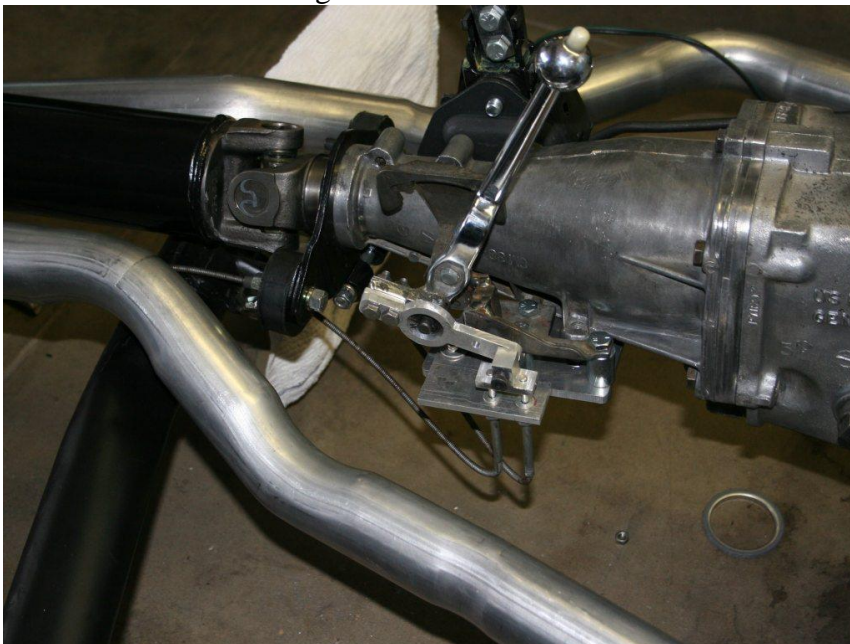
Exhaust cut out control mounted to the transmission side. Cables used to control the cutout.
