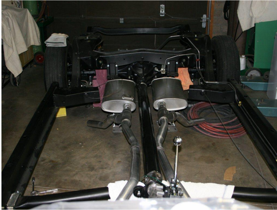
Exhaust with cutouts near mufflers.
