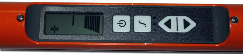
The Magnastick MSL Magnetometer seeks ferromagnetic objects by sensing their magnetic fields. Dual sensors detect the magnetic lines of flux naturally present in ferrous (iron) materials and are not affected by non-ferrous materials such as brass, aluminum, or copper.
