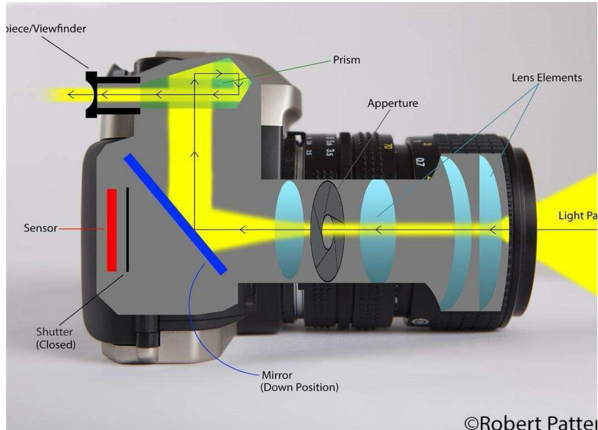
The shutter is the **BLACK** device (in front of the **sensor**) that opens allowing light to reach the sensor when the **mirror** is up and shutter button is pressed.
