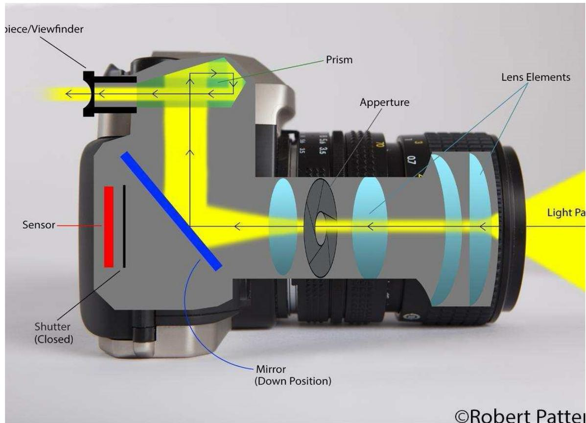
In **Live View**, the **BLUE mirror** stays flipped up so the light reaches the **sensor** and the image is projected directly on the LCD screen.
