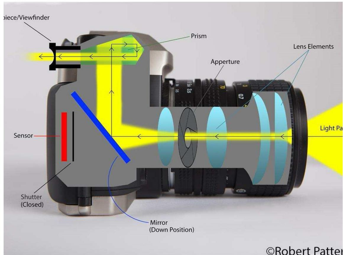
Note that, on most cameras, the image is eventually focused on the **Prism** which you see in the Viewfinder. It doesn't matter if the image is of something 2 feet in front of the camera or at infinity. It's **always** focused on the prism.
