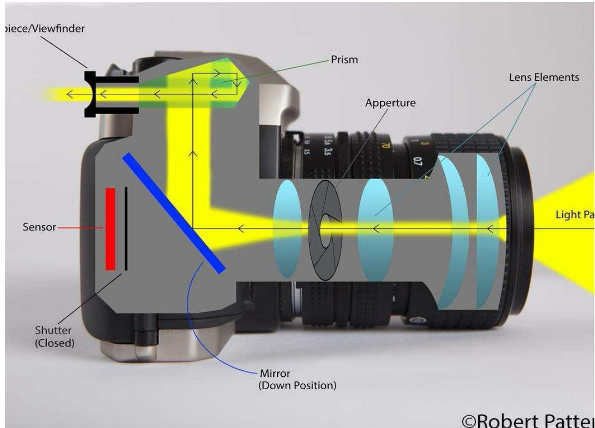
The **mirror** is the **BLUE** device (in the camera) that directs light to reach either the viewfinder or the sensor. To allow light to reach the sensor, the mirror has to flip up when the shutter button is pressed.
