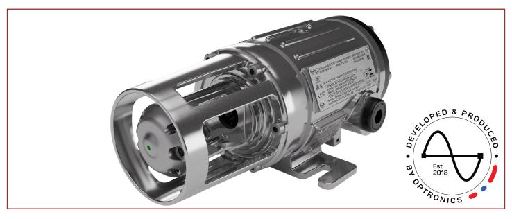
The Optronics PG11 is an explosion proof, rugged Optical Hydrocarbon Gas Detector. PG11 comes with a life-time factory calibration, is easy to install and commission and has very limited need for maintenance. The Solid State Infrared SafeSource™ ensures unmatched stability and lifetime and the built-in condition monitoring keeps maintenance and process abruptions at a minimum. Any need for attention is automatically informed to the operator.
