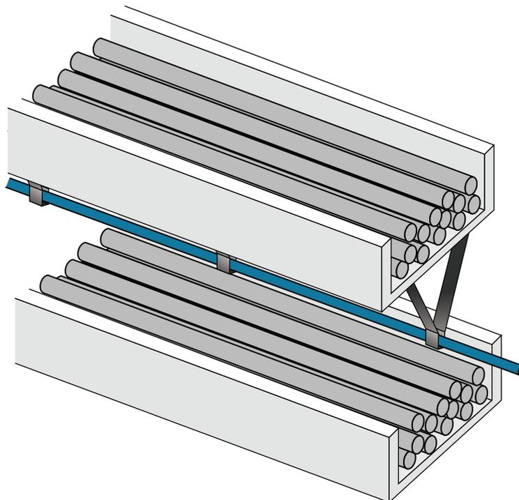
Figure 5: Protecting multiple cable trays using LHD cable
