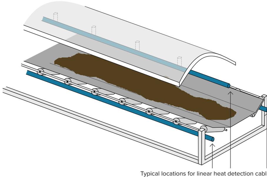
Figure 6: Typical locations for protecting conveyors with LHD cable
