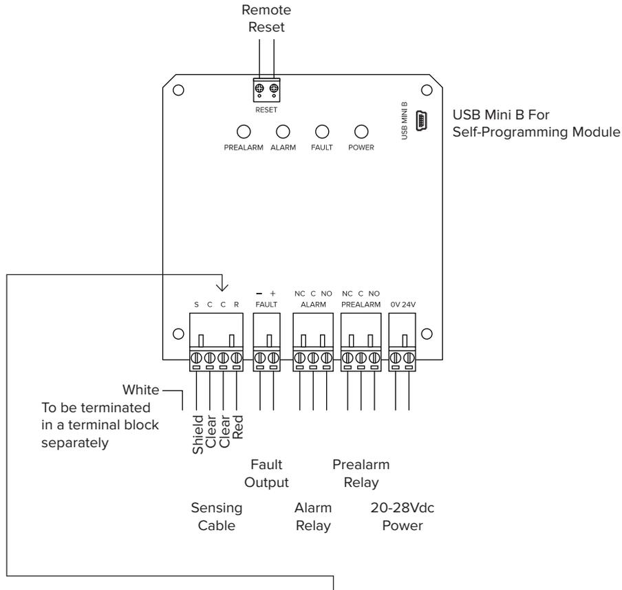
The clear cores are polarity sensitive once the End of Line module has been terminated. Ensure that the clear cores have been terminated correctly by following the steps below:
