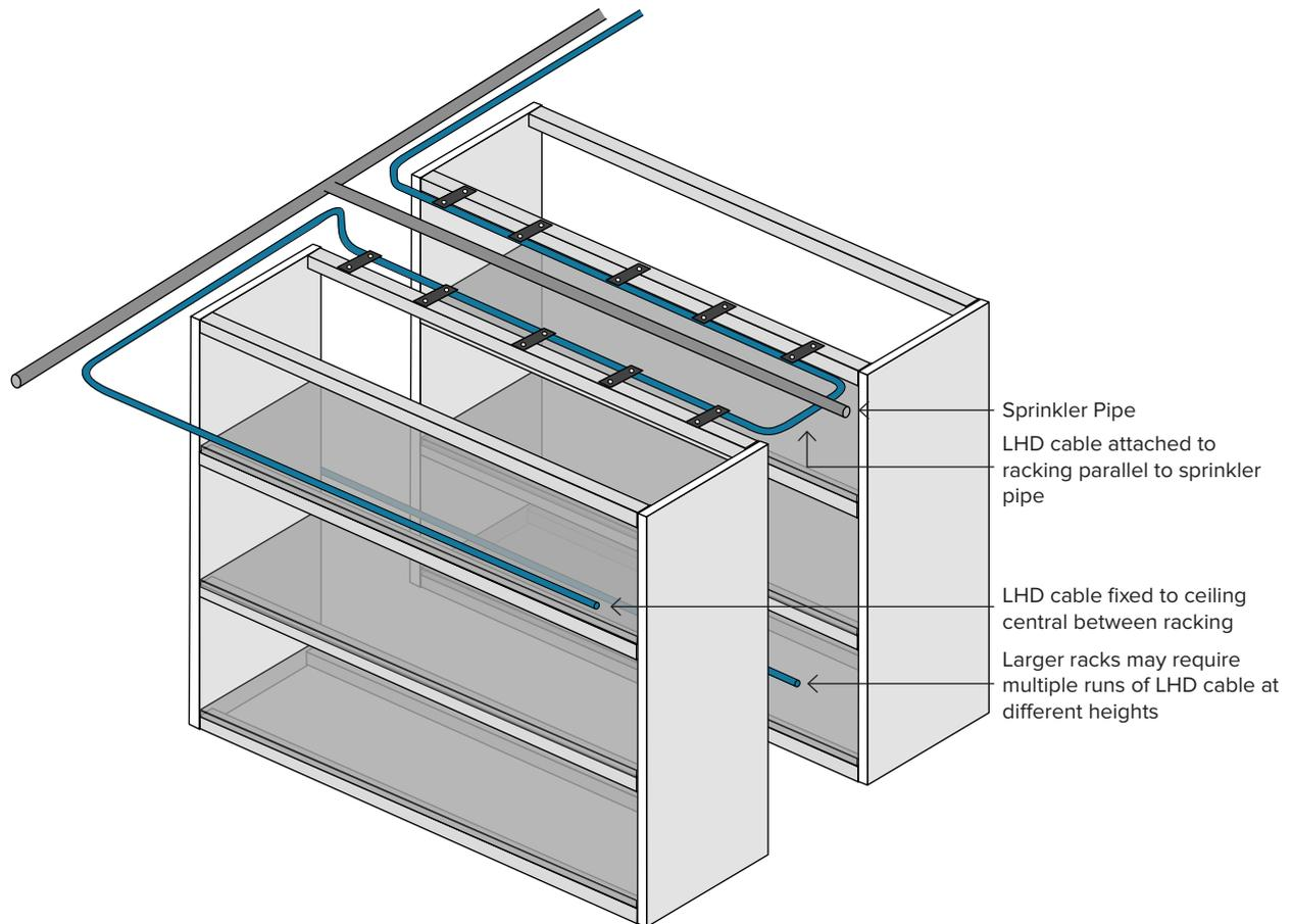
Figure 7: Typical locations for protecting racked storage with LHD cable
