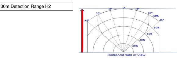
1. H2 Detection Field of View test Methane and Syngas
