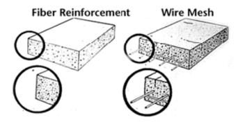
In its plastic state, Nycon-reinforced concrete has more flexural (tensile) strength and toughness to ductility fracture; it has increased impact resistance, fatigue life, thermal-shock resistance, and abrasion resistance. With the length, width, and frequency of cracks reduced, there is lower water migration, less permeability and volume change. Finally, fibers are non-corrosive, non-abrasive, rustproof, and that means less spalling because of oxidation and steel corrosion.
