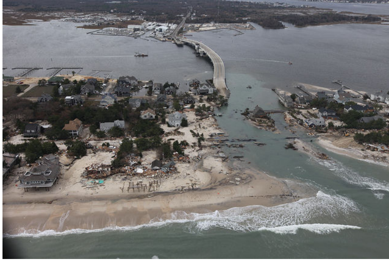
Figure 19 Aerial photo of Mantoloking, NJ breach following Sandy. NJ State Route 35 is destroyed (left to right in middle of photo) where the ocean meets the bay at the Herbert St. (Ocean County Route 28) bridge (G. Thompson, US Fish and Wildlife Service)
