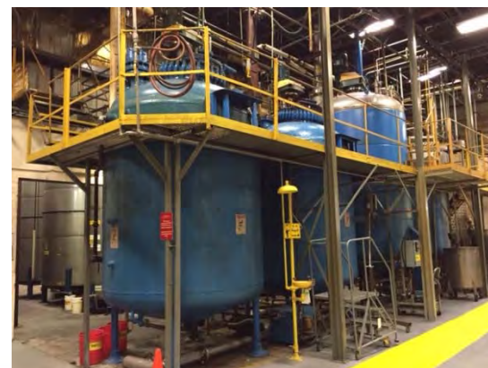
Acrylic Polymer Reactors
