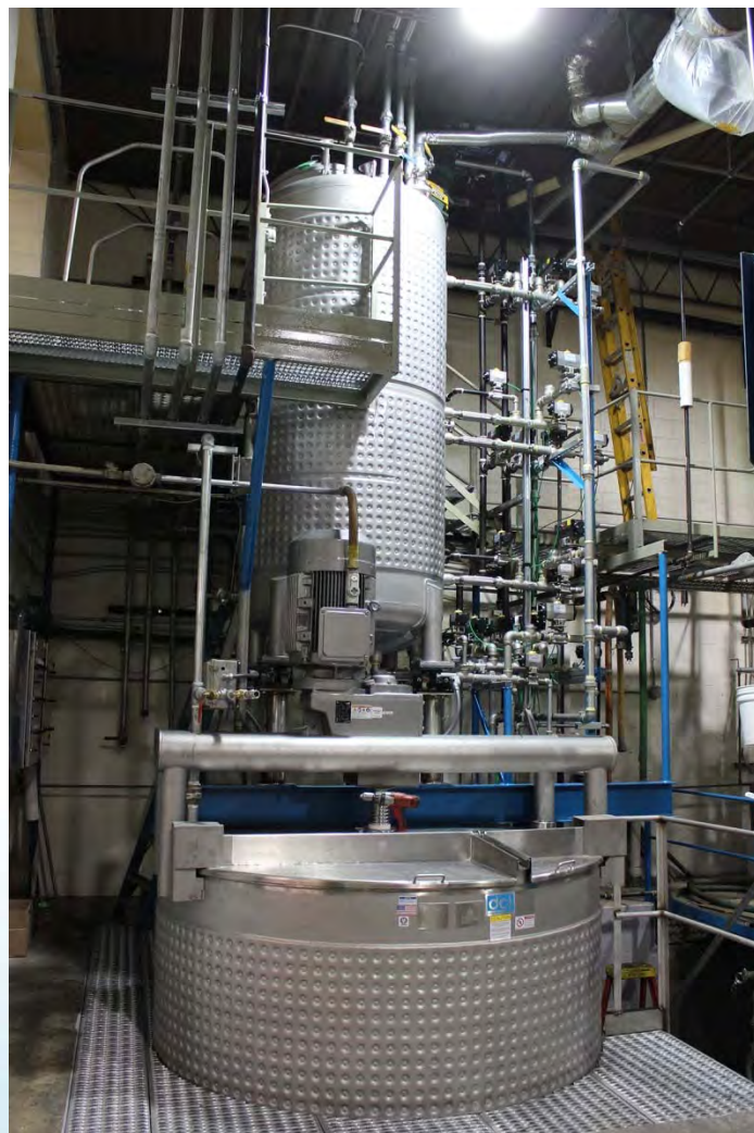
Acrylic Polymer Reactors
