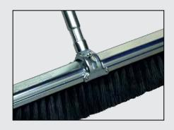
No other brush comes close to matching the unique features of the Speed Sweep® system. A steel back is placed over the brush block and crimped permanently onto the block. Steel rivets are fastened through the entire block to secure the adjustable steel socket.
