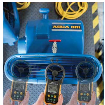
CFM is calculated by averaging measurements at the center and the outer edges of the vent.
