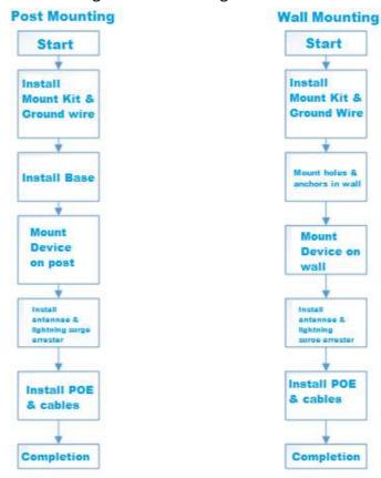
Figure 6 Diagram of Equipment Installation Procedures
