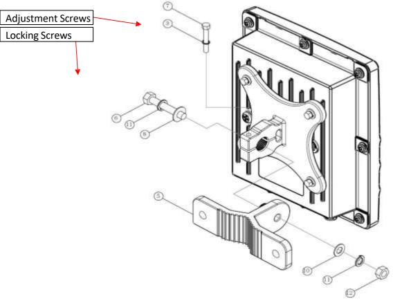
Figure 8 Assembling the Base Frame - Diagram II
