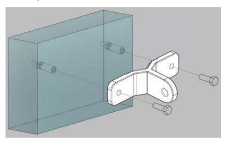
Figure 13 Installation Diagram of Adjustable Plate
