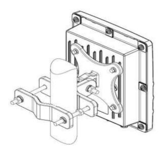
Figure 10 Diagram II of Pole Installation
