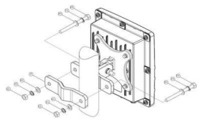
Figure 9 Diagram I of Pole Installation
