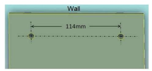
Figure 11 Width between the wall mounting holes
