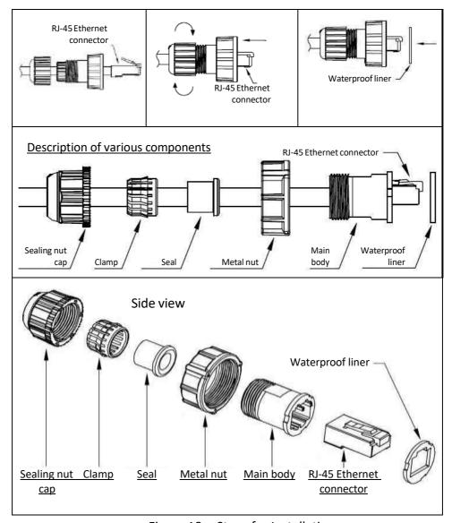
Figure 18 Steps for Installation
