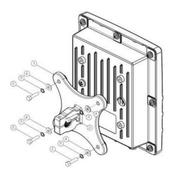
Figure 14 Assembling Diagram of Base Frame
