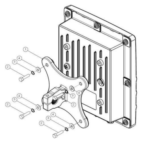
Figure 7 Assembling the Base Frame - Diagram I
