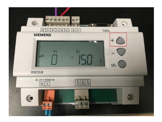
To adjust the heating setpoint, press the '+' button until 'SP-H' is on the screen
