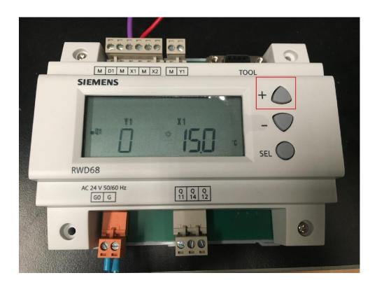
To adjust the cooling setpoint, press the + button until 'SP-C' is on the screen
