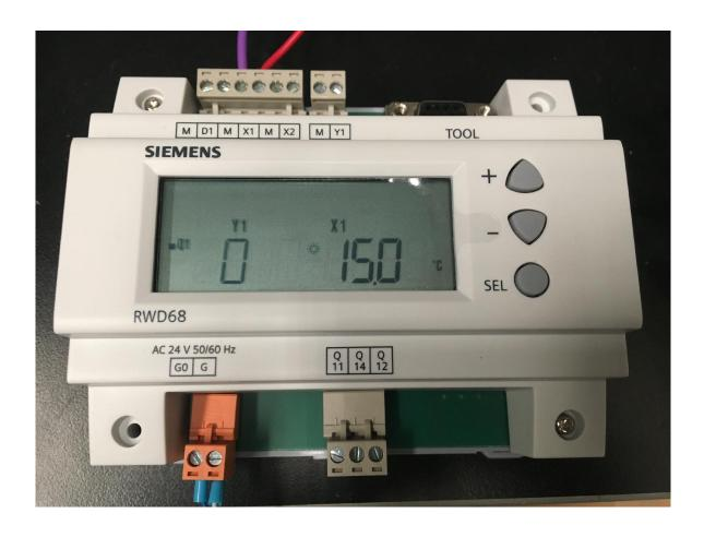
X1 Value is the current room temperature Y1 Value is the cooling signal, 0=no cooling signal, 10=maximum cooling signal Q1 is the Electric duct heater status
