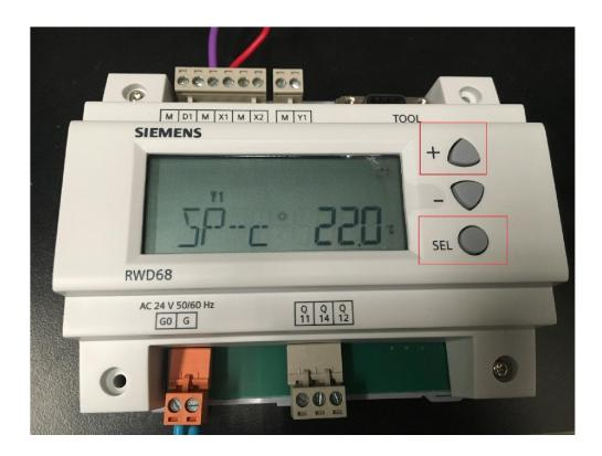
Press 'SEL' button, the number value will flash, adjust to desired value using + or – buttons. Press 'Sel' button to confirm selection.
