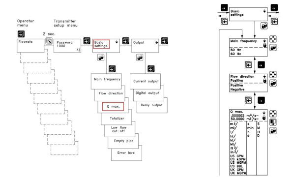
3. Change the Qmax value <u>including the units</u> to be 10-20% above that of the maximum expected flow rate though the Magflo meter. If the maximum value is unknown a temporary rule of thumb flow rate can be used (see table below). Change the Qmax value once the maximum flow rate is determined or provided.
