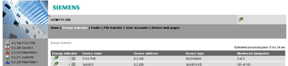
The screenshot shows the Siemens web interface for plant OZW772.250. The primary navigation bar includes 'Home', 'Energy indicator', 'Faults', 'File transfer', 'User accounts', and 'Device web pages'. The 'Energy indicator' function is selected. Below the navigation bar, a table displays the energy indicator data for two devices:
