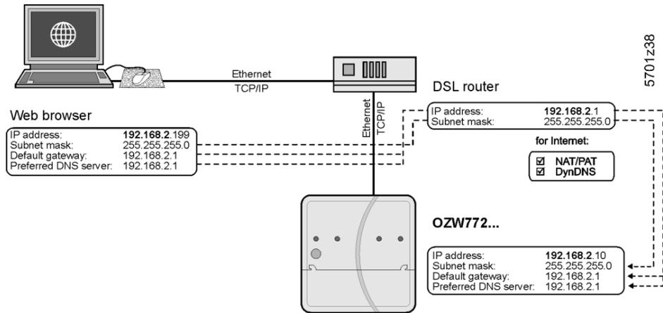
A router normally serves as the DHCP server if installed on a local area network (e.g. DSL router for Internet access). As such, it automatically assigns IP addresses to all participants that are DHCP clients.
