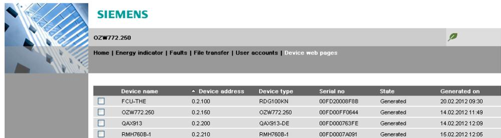
The screenshot shows the Siemens web interface for plant OZW772.250. The secondary navigation bar includes 'Home', 'Energy indicator', 'Faults', 'File transfer', 'User accounts', and 'Device web pages'. The 'Device web pages' pane is selected, displaying a table of devices with their status and generation time:
