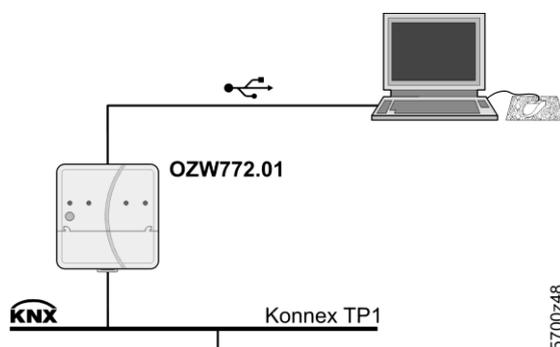
4. The RNDIS driver is installed automatically if the PC is connected to the Internet and no RNDIS driver is installed as long as the Microsoft online update is enabled. Follow the instructions for the installation program.
