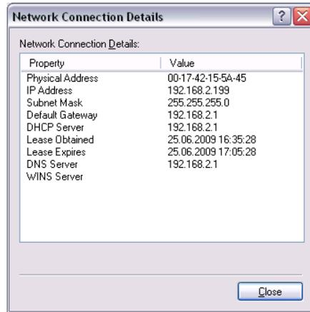
In the example, the PC is assigned the IP address [192.168.2.199](#) and subnet mask [255.255.255.0](#). The default gateway and DNS server have IP address [192.168.2.1](#).
