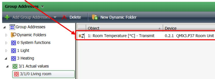
An available 2-byte data point is required to display a temperature in OZW. It is select from the ETS device list under "OZW772 web server" and defined.
