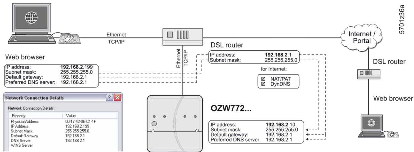
The illustration shows a typical application with operation via Internet and home network. Use can use "Network connection" to issue IP address, subnet mask, standard gateway and preferred DNS server if the PC is connected to the home network.
