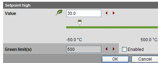
The screenshot shows a dialog box titled "Setpoint high". It contains a "Value" field with the number "30.0" and a green leaf icon to its left. Below the value field is a horizontal slider bar with a green track and a white knob. The range of the slider is from -50.0 °C to 500.0 °C. Below the slider is a "Green limit(s)" field with the number "500" and a disabled checkbox labeled "Enabled". At the bottom of the dialog are "OK" and "Cancel" buttons.
