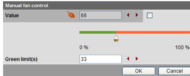
Dialog boxes for data points with a manually set value contain a checkbox. The value cannot be entered manually if the checkbox is cleared . The entry field and the arrows ◀ ▶ are grayed and the "Value" slider is hidden.
