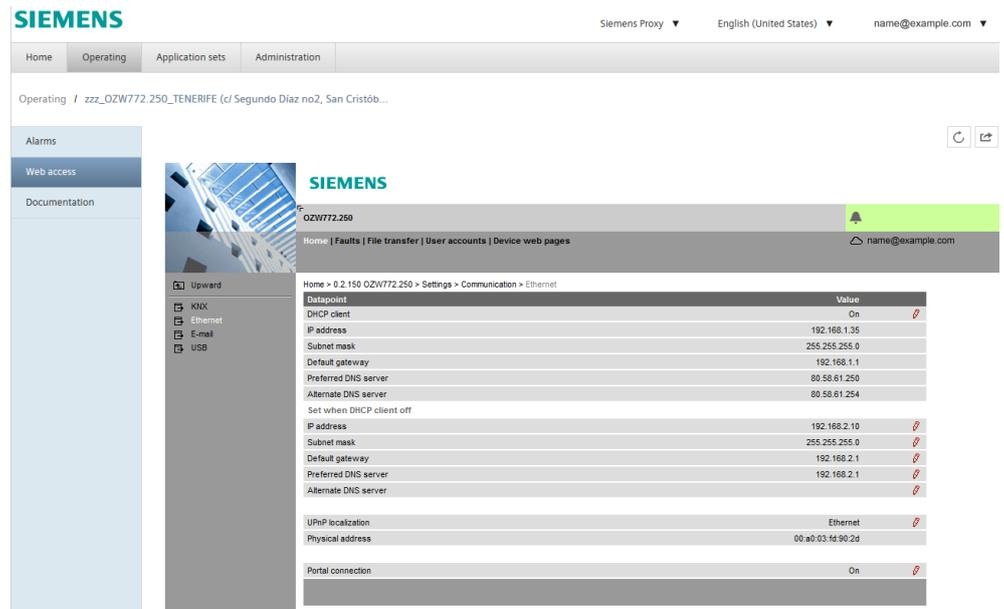
The screenshot shows the Siemens OZW772.250 web interface. The top navigation bar includes 'Home', 'Operating', 'Application sets', and 'Administration'. The 'Operating' menu is active, showing a list of plants. The 'Web access' button is highlighted. The main content area displays the network configuration for the selected plant, including a table of network parameters.
