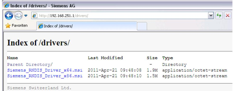
The driver [Siemens\\_RNDIS\\_Driver\\_x64.msi](#) is installed on a 64-bit operating system; on a 32-bit operating system [Siemens\\_RNDIS\\_Driver\\_x86.msi](#). The installation file for the driver can be executed directly on the PC. Following the steps for the installation wizard.
