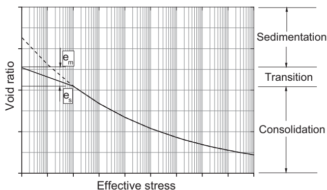
Fig. 4. Schematic of void ratio versus \log_{10} effective stress sedimentation and consolidation [3].
