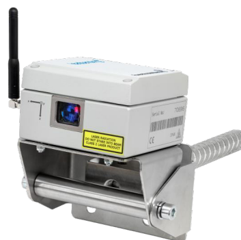
Fig. 5: LaserTilt90 mounted on a swivel mounting bracket LS-ACC-LAS-SB that includes the attachment option of a convergence bolt with a G3/8" male thread.
