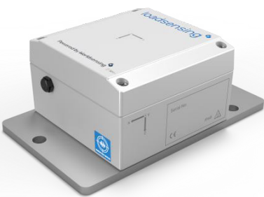
Fig. 3: Versatile horizontal surface mounting plate (LS-ACC-IN15-HP), recommended for both horizontal and vertical mounting. The plate has three clearance holes for M8 anchor rods and an M8 threaded hole available for installing a monitoring prism or a button head screw for precise levelling.
