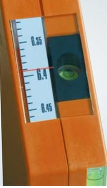
The height of the laser plane can be read off from the analogue display easily.
