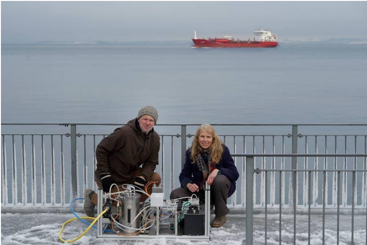
Nick Blackburn (CTO at MicroWISE and Pia Haecky (CEO) with the BallastWISE Inline robot for installation on board of vessels or in conjunction with shore-based ballast water treatment systems, at the Port of Aarhus, Denmark.
