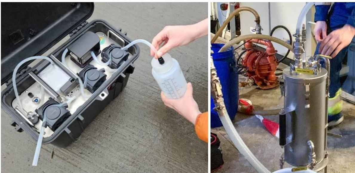
BallastWISE portable CMD (left), and the BallastWISE Sampler during shipboard test (right).
