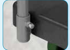
Steel outside deck handle pockets are welded to under deck reinforcements. Jam bolts, standard on all models, hold handles in place
