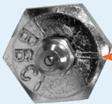
Grade marking opposite manufacturer IS points to the same side as the exit hole on the shaft.
