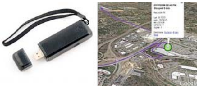
TrackStick, a $200 GPS lifelog the size of a pack of gum
