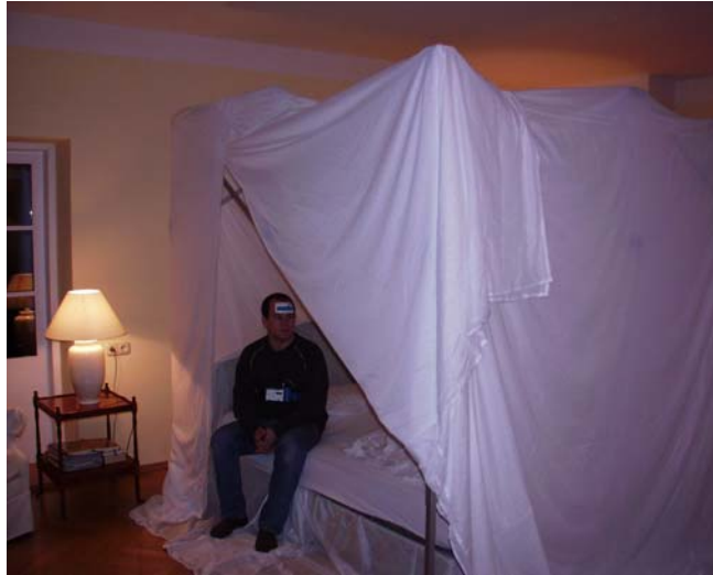
Figure 2 Mobile EF shield around the bed and proband with somnomedical data acquisition means.
