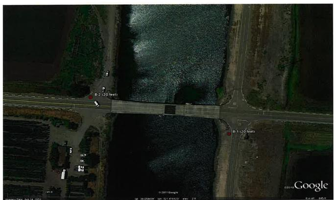
The subsurface conditions at the site will be explored by drilling one boring at each approach embankment location (2 borings total) to the following depths:
