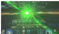
1. Hit the transponder identification button as soon as pilots are aware of being lased. This will mark the plane's position on the air traffic controller's radar scope, which may help law enforcement triangulate where the laser light is originating from.
