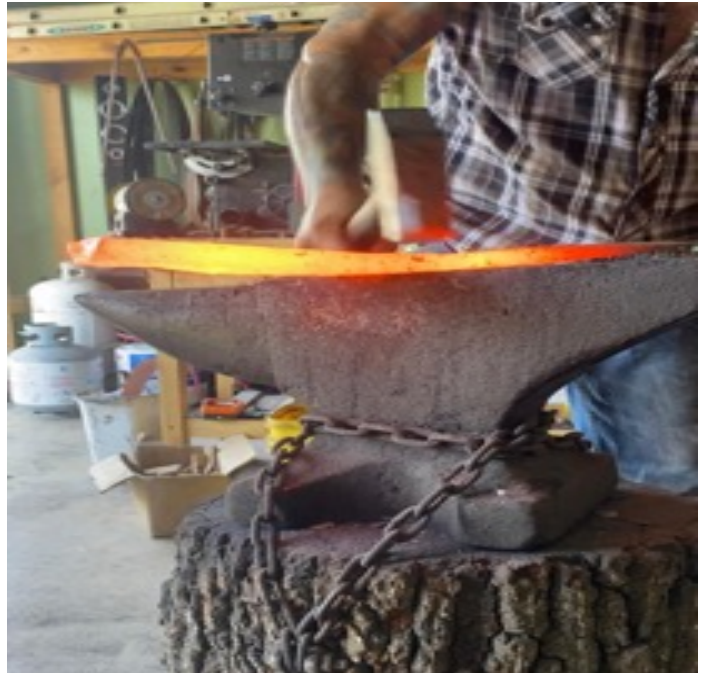
Early stages of forging Oso Naval Lodge No. 1282 Tiler's sword made from 68 Camaro leaf spring.
