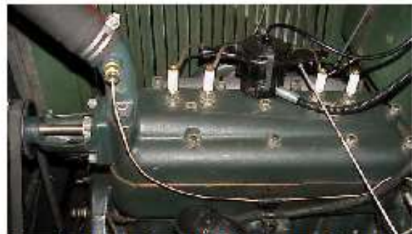
The six-foot mechanical cable is routed from the gauge to the Dan Eubanks reproduction water outlet casting that has been cast with a temp gauge boss and has been drilled and tapped for your favorite size pipe fitting. Dan locates the fitting on the side of the casting to accommodate an overhead valve head installation. (Dan Eubanks 626-827-4004).
