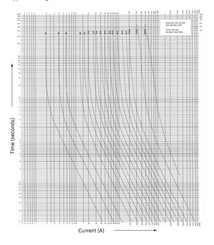
Type T Melting Time-Current Characteristic Curves
