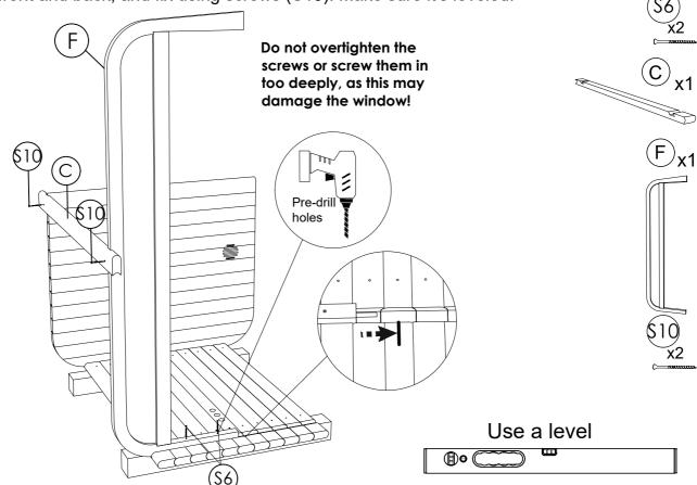
**STEP 8**: Place the second front panel (F). Slide it together that the top and bottom connects. Fix it at the panel threshold with screws (S6) pre-drill holes. Make sure it's level. Use metal bracket
