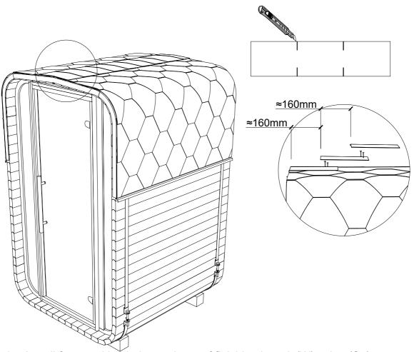
**STEP 34:** Install front and back decorative roof finishing boards(W) using (S7) screws. Start by fixing one bottom board. Draw a center line put board exactly in the middle. Fix it about 5mm above floor boards, then rest of the boards goes next to each other.
