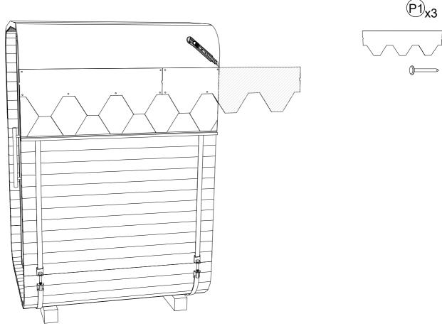
**STEP 30:** Third row goes exactly like first row. Cut half of hexagonal part from shingle and fix it with shingle nails. Remove protective film from the bottom of the sheet.
