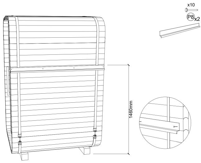
**STEP 26**: Lay out underlay on both sides first. Than lay middle part on top of the roof, that it is evenly placed and covers both underlay sheets. Leave about 40mm over the front and back edges. Staple underlay at the front and back edges. Cut excess underlay if necessary.
