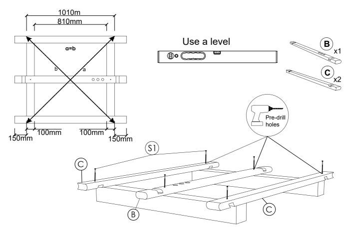
**STEP 2:** Attach five staves (C) on each side of the center stave. Check the level while installing the staves and use a rubber hammer for a tighter fit. Pre-drill holes for the screws. After fixing eight staves, remove the side staves and reattach them.
