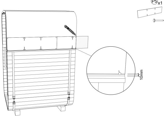
**STEP 28**: For 1st shingle cut off the half of hexagonal part. Remove protective film from the bottom of the sheet. Start placing shingles over starting shingles. Fix 2nd shingle needs to be cut. Measure the necessary length and fix it with nails.
