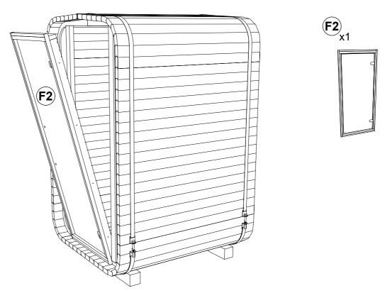
**STEP 17:** Put plastic spacers in the gap between the door box and the front panel where the screws go. Combine spacers for best width. Spacer must fit tightly.
