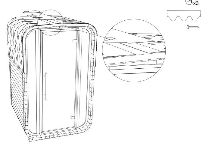
**STEP 33:** For top of the roof use starting shingles. Cut some shingles in squares, there are marked lines. Take off protective film. Nail each shingle with two nails. Next shingle goes about 160mm over previous. After it's done, use heat source for better adhesion.
