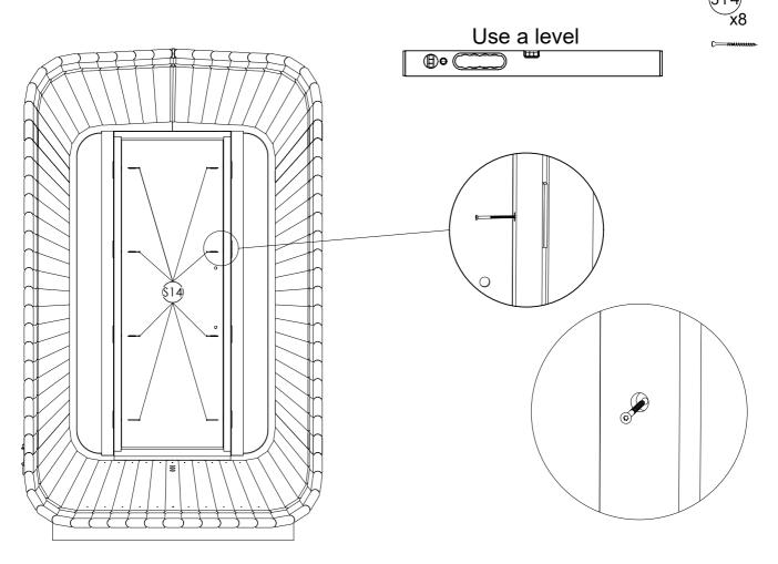
STEP 19: Fix door moldings to both sides and on top of the door with (S5) screws.
