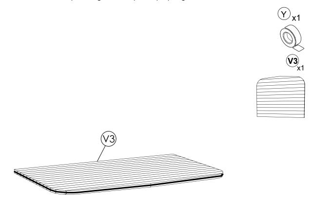
STEP 11:Install the panel (V3) with caution. Use spray foam between panels for better insulation. Place it on top of the lower back panel (V). Check level and that side edges are aligned with bottom panel. One keeps holding the panel, and the other is fixing the side stave on a upper curve using screws (S10). Secure the panel (V3) at the both corners using two screws (S4).
