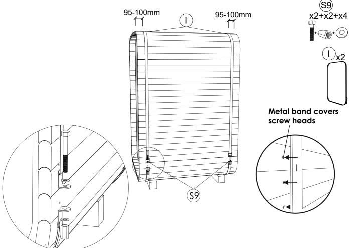
**STEP 16**:Install the doors (F2). Put the doors on threshold and lay in frame about in the middle. Fix doors with clamps or another person should hold the door.
