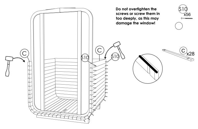
**STEP 10**: Attach adhesive tape along the rear panel (V3) edge.
