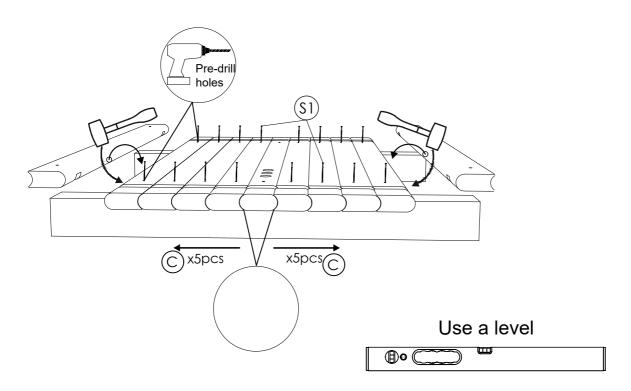
**STEP3:** Drill ten 10mm holes in front and back wall grooves to the out-side in board connections as shown in the picture. This will help drain excess water faster - **Optional**.
