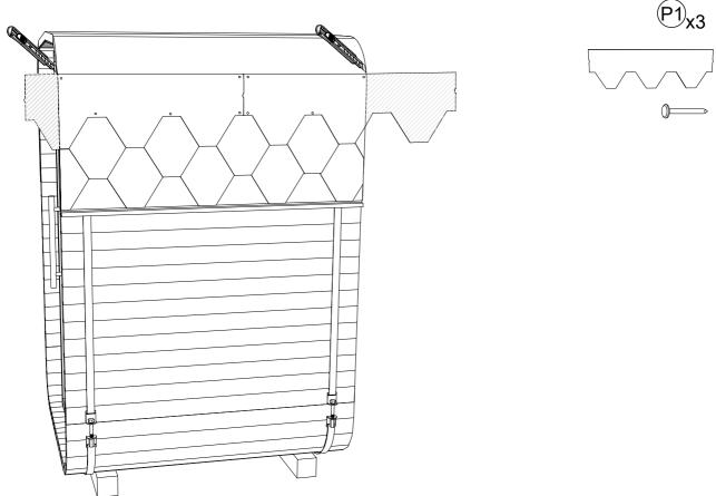
STEP 31: Keep placing shingles till last layer goes over the middle of the roof.
