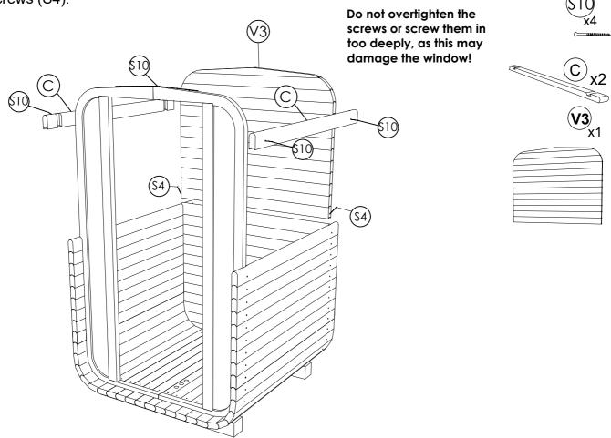
STEP 12: Fix 17 staves (C) on both sides with screws (S10). Use rubber hammer for tighter placement. Keep fixing staves till reach top of the roof.
