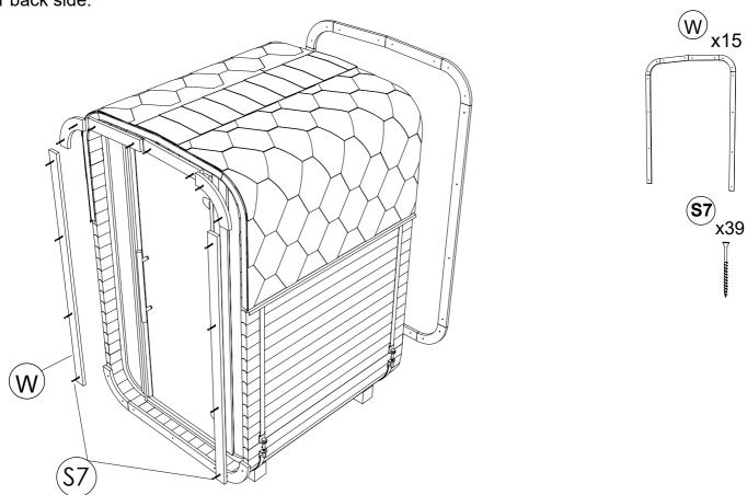
**STEP 36:** Use sillicon sealant behind decorative boards to fill gap between shingles and boards at the front and back side.
