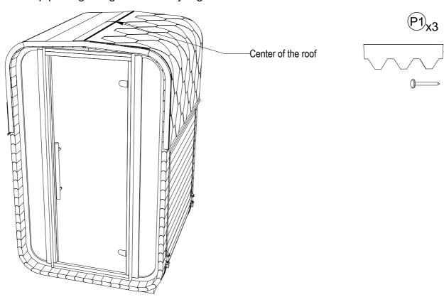
**STEP 32:** Repeat same steps for other side, till last layer goes over middle of the roof. Use heat source for better adhesion. Lift every rectangle, heat a bit with some heat source and press it to the roof.
