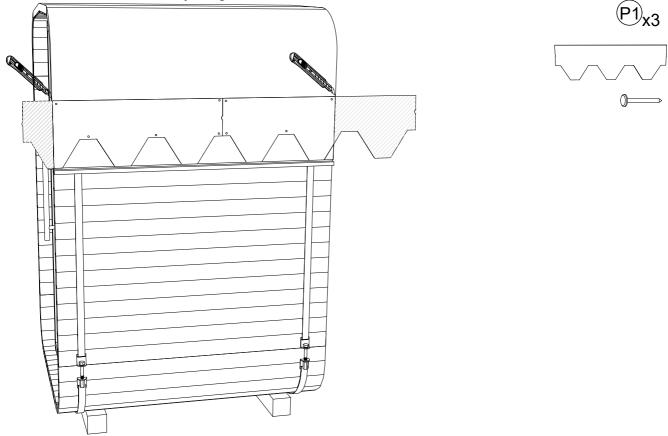
**STEP 29:** Remove the protective film from the bottom of the sheet. The second row starts with the whole shingle, fix it with shingle nails. Last shingle needs to be cut by measured length.
