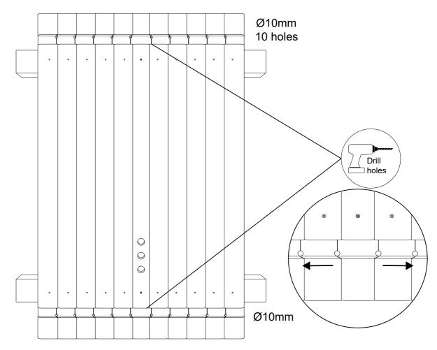
**STEP 4**: You may attach adhesive tape along the rear panel's edge. At the bottom of the rear panel (V), draw a line where the centre of the panel is. Do the same on the centre stave of the floor, where the panel will be sitting **(optional)**
