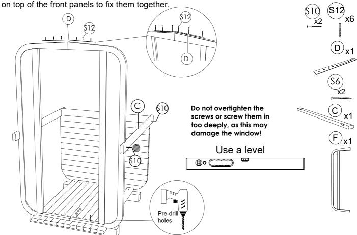
**STEP 9**: Fix 14 staves (C) on both sides with screws (S10). Use rubber hammer for tighter placement. Keep fixing staves till reach top of the rear panel (V).
