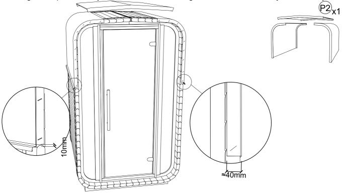
**STEP 27**:Remove protective film from the bottom of the sheet. Place starting shingles next to each other. Then fix with nails as in picture. Cut excess part of the starting shingle before nailing it. Do the same on the other side.
