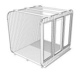
(9) The stave covering the lower fillet needs to be fixed with screws.
