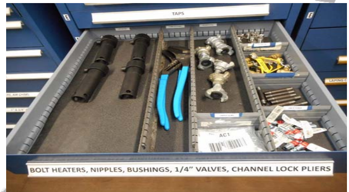
Bolt Heating Tooling
