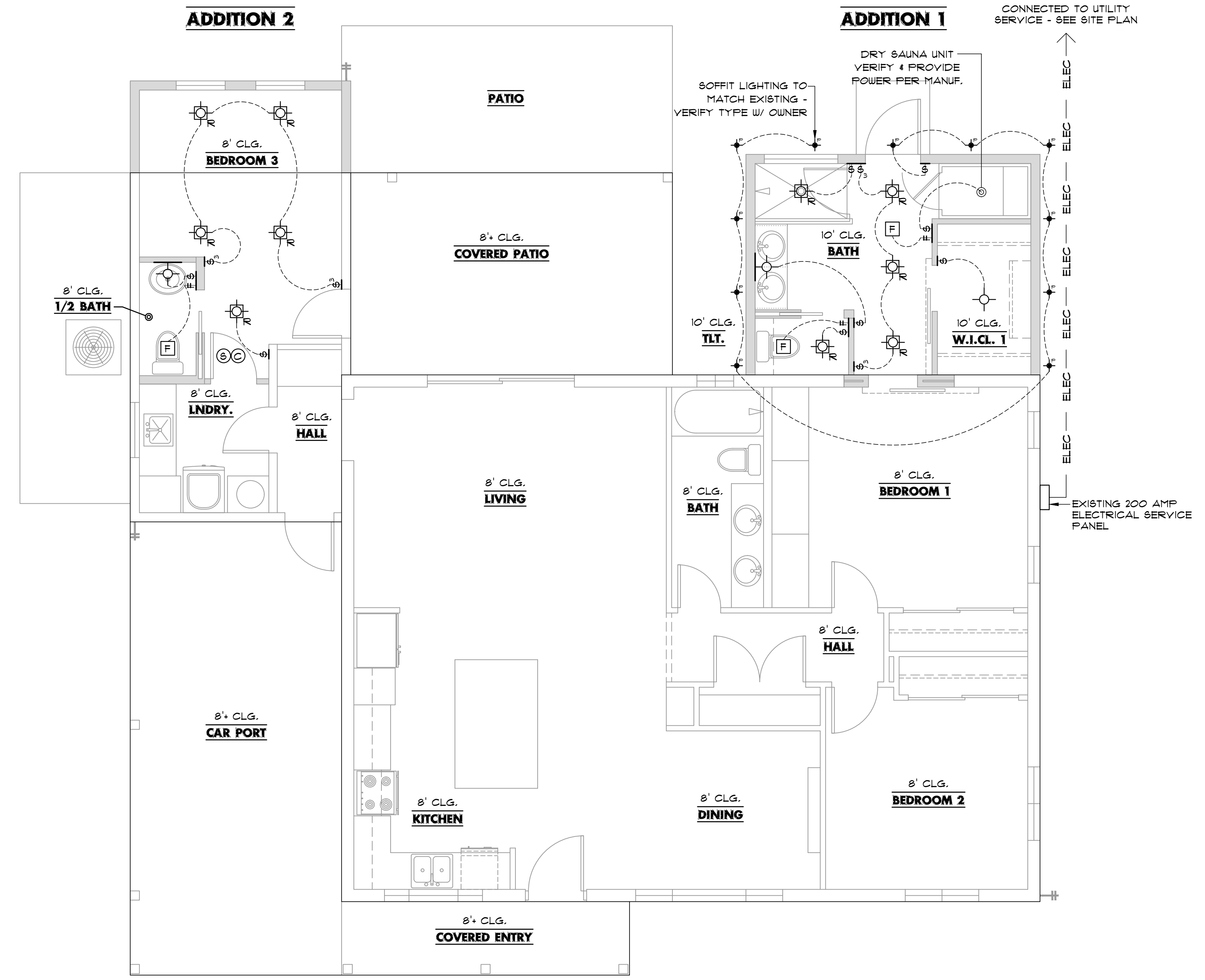
SCHEMATIC ELECTRICAL LIGHTING PLAN SCALE: 1/4" = 1'-0"
