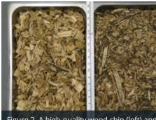
Figure 2. A high-quality wood chip (left) and a lower quality wood chip (right).
