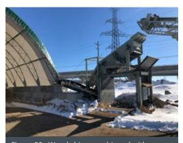
Figure 29. Wood chips are chipped with conventional, hand-fed chippers and then screened with a three-deck aggregate screener to filter out fine and coarse particles, leaving only chips of the appropriate size for the bioheat system. (Photo: Biothermic)
