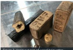
Figure 3. Various types of wood briquettes. (Photo: CanmetENERGY, Natural Resources Canada)
