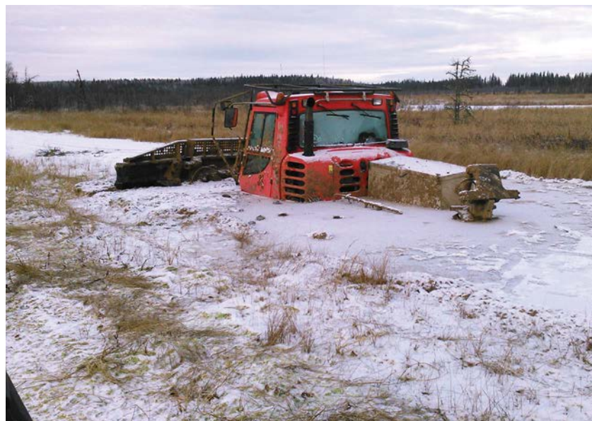
FIGURE 11. Example of equipment submerged in a peatland. Understanding wetland type can provide information about potential peat depth and subsurface water flow, important considerations for making safe decisions when operating in and around wetlands. Photo courtesy of Millar Western.
