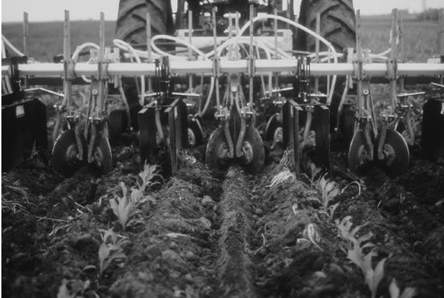
FIGURE 8.8 One of the custom-made tillers used for cultivation of the ridge-till systems on the Thompson Farm in Boone, Iowa. The tiller is completing the first cultivation pass after planting of the corn crop, in which soil on the shoulders of the ridges is cut away (killing weeds) and then pushed back. Dick Thompson pioneered the ridge-till system in the 1980s, after recognizing that even though conventional cultivation killed weeds, it also created the ideal disturbed environment for their regrowth. Over the years, thousands of farmers and researchers visited the Thompson Farm to learn from the acknowledged “expert” on ridge-till systems.
