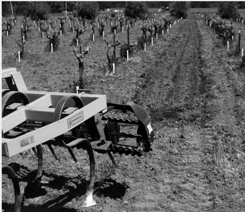
FIGURE 6.6 A special harrow used to create the dry-farm dust mulch. A uniform layer of dry soil on top of the moist soil below breaks capillarity and reduces evaporative moisture loss.
