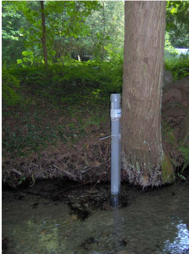
Figure 1: Crest stage gauge attached to both rebar and a tree
