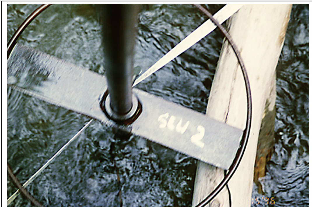
Figure 21: Cover Ring (30 cm in diameter), Showing the 'Observation Area'.
