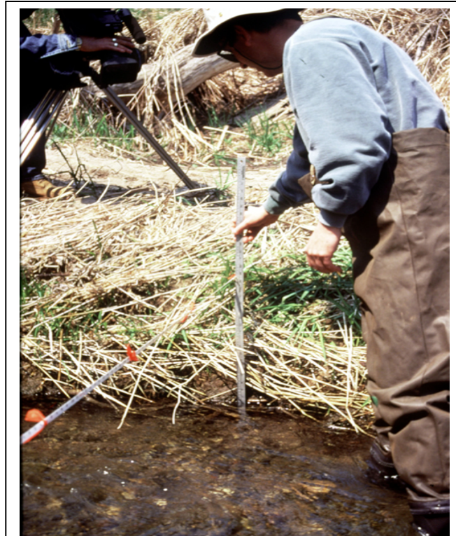
Figure 6: Measuring Height from Channel Bottom to Tape at the Active Channel Boundary.
