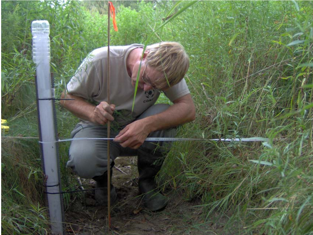
Figure 1: Conducting a bankfull profile at a crest stage gauge within a headwater stream
