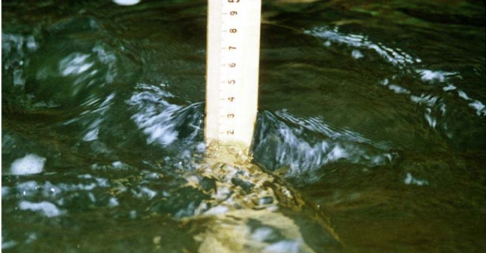
Figure 4. A point measurement of hydraulic head.
