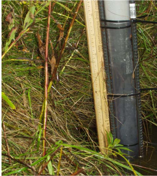
Figure 3: Example of Crest Stage Gauge with response
