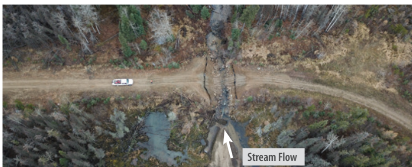
Aerial view of a successful reclamation of a wetland crossing. The culvert was removed, and the stream bed was restored.
