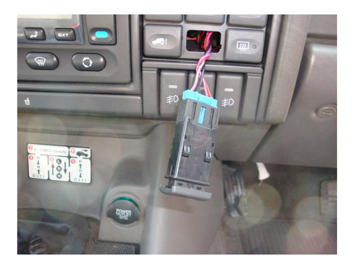
**C.** Once the Facia Switch is unplugged from its Blue Connector, you will need to carefully remove the Wires and Terminals from the Blue Connector. *(see D. and Annex to this document)*
