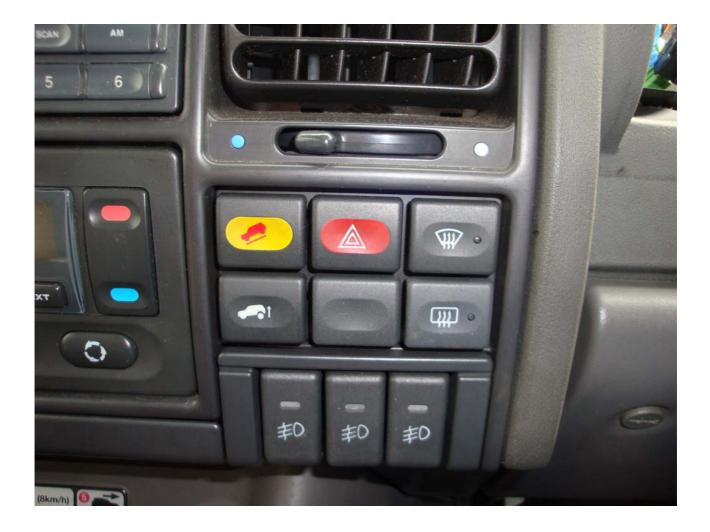
The position occupied by the original fuel flap release switch can now be used for another switch from a Discovery II, Freelander 1, or post-2002 Defender.
