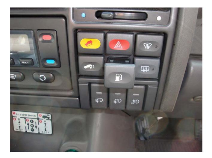
B. Un-plug the Blue switch connector from the switch –
