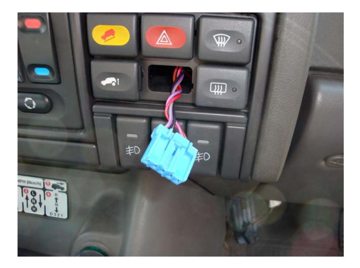
**D**. Remove the terminals from the fuel flap switch's Blue connector and insert them (in the correct order) into the White female connector supplied with the Relocation Harness –
