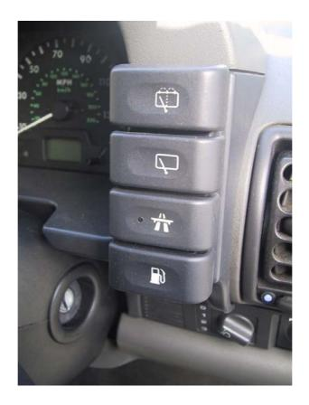
Fit the instrument cowl onto it's two facia clips and replace the 2 x screws.
