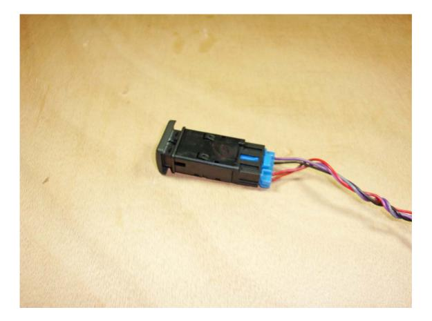
ii. Press release tab on Blue switch connector
