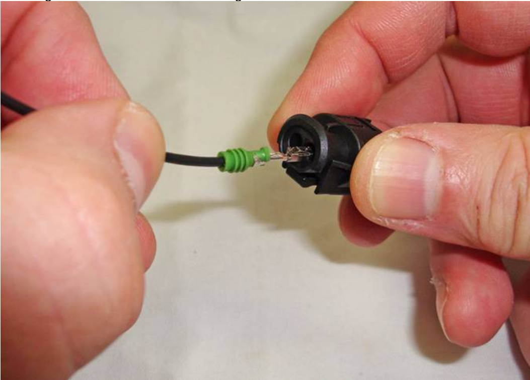
Inserting terminal into connector housing
