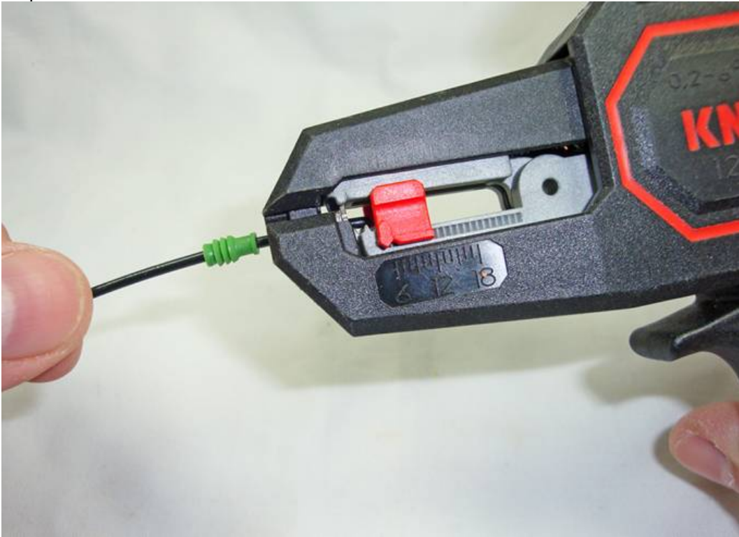
Strip insulation from cable
