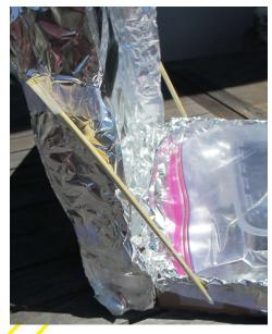
How it Works: Rays of sunlight do the heating. Some rays go through the clear bag and clear lid, to be absorbed directly by the food, converting the infrared light energy into heat energy. Some rays strike the black food tray and are absorbed by the dark-colored material, warming the tray by converting the infrared light into heat. Some rays are reflected by the foil towards the food, increasing the amount of solar radiation striking the food.
