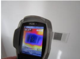
The system did not operate within the allowable tolerances. The air coming out of the vents should be 14 to 21 degrees cooler than where it goes into the cold air return. It is recommended that a qualified contractor be consulted regarding this matter.
