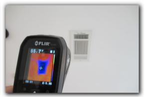
The air coming out of the vents should be 14 to 21 degrees cooler than where it goes into the cold air return. These readings are within the recommended tolerances for proper operation.
