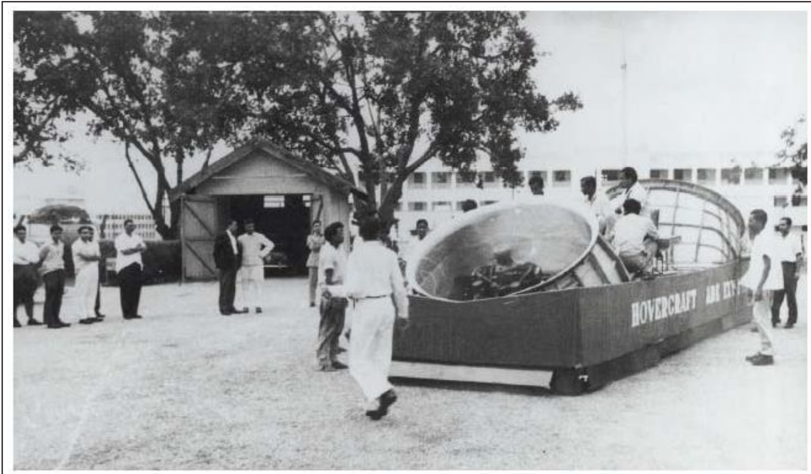
Plate 9 The twin-engine indigenous hovercraft prototype Nandi developed at ADE, Bangalore. As inventor and pilot, I took my rightful place at the controls.
