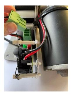
2 - Unplug the wiring from the side of the winch unit
