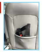
Disconnect the winch attachment from the wheelchair and the winch unit, and store it somewhere safe and secure. Ensure the front restraints are still attached to the wheelchair correctly. Then fit the remainder of your restraint system, referring to your restraint handbook for more information should you need to.
