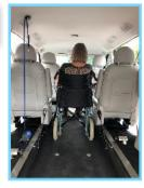
Use the 'IN' and "OUT" buttons on the winch remote as necessary, until the wheelchair is positioned correctly inside the vehicle.
