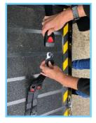
Click the wheelchair attachment (either T bar or Y harness) onto the end of the winch belt.
