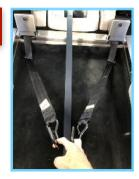
Guide the restraint belts out of the vehicle, down the ramp and attach them to the wheelchair frame. Once attached, press the switch again to lock the restraints from further release.
