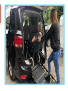
Move behind the wheelchair and hold the handles. Press the 'IN' button on the remote control and slowly enter the vehicle. It is important to remain behind the wheelchair for guidance at all times.
