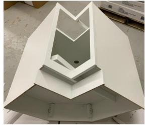
Tilt cabinet onto its back and attach the toe kick. You can also use this position to get easier access to hard to reach areas.
