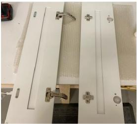
Attach hinges and magnet pieces to the doors, then connect doors together.
