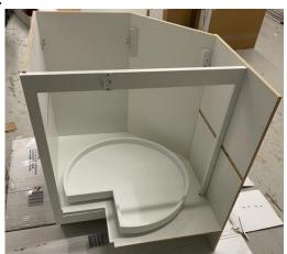
Set the frame into the notch on the bottom shelf.
