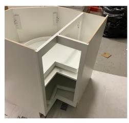
Attach the second face frame piece ensuring the side panel fits fully into the groove.
