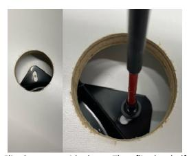
Flip the tray upside down. Then flip the shelf upside down. Using the hole you cut previously, line up the holes in the hardware with the predrilled holes in the tray. Partially attach the screw, rotate the hardware and repeat. Once all four are partially screwed in, go back and fully fasten the screws.
