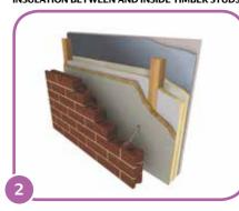
to prevent the insulation boards from moving and provide the specified air cavity within the frame if required. This cavity may be used as a service void.
