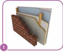
Eco-Versal can be installed inside the timber studs in addition to between them to reduce the cold bridging effect and further improve the thermal performance of the wall. Insulated plasterboard such as Eco-Liner can be used as an alternative inside the timber studs helping to reduce installation time. When fixed to timber framing, the maximum board span should be 600mm. The insulation board must be installed flush with the stud and there should be no gap between insulation layers.
