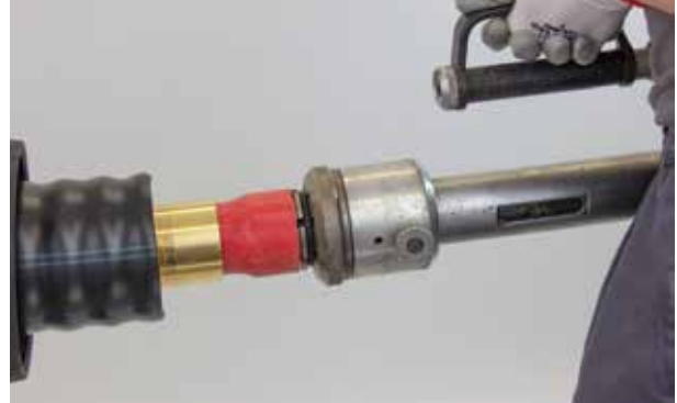
(2) Expand the pipe end twice – offset by approximately 30°. Ensure that the compression sleeve is slid well back from the area being expanded.
