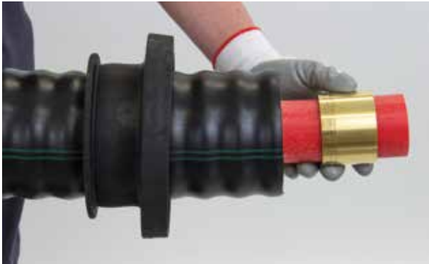
(1) The PEX-LOK compression sleeve can be slid onto the prepared pipe ends. The square end faces the insulation and the chamfered end faces towards the joint.
