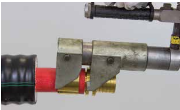
(3) Insert the PEX-LOK fitting (tee, elbow or straight coupling). Locate the clamping jaws on the tool and clamp onto the joint. For dimensions over 40mm, a lubricant of petroleum jelly must be used in the area of the compression sleeve.
