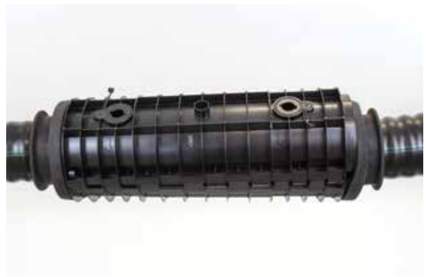
(2) Position the upper half of the shell sleeve over the lower half, taking care to align the longer catches (as ringed on the photograph). Also ensure that all joining faces of the two shell halves are clean.
