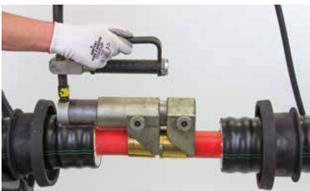
(5) Clamp the second pipe. If this is a straight or 90 degree coupling, then the connection is completed.
